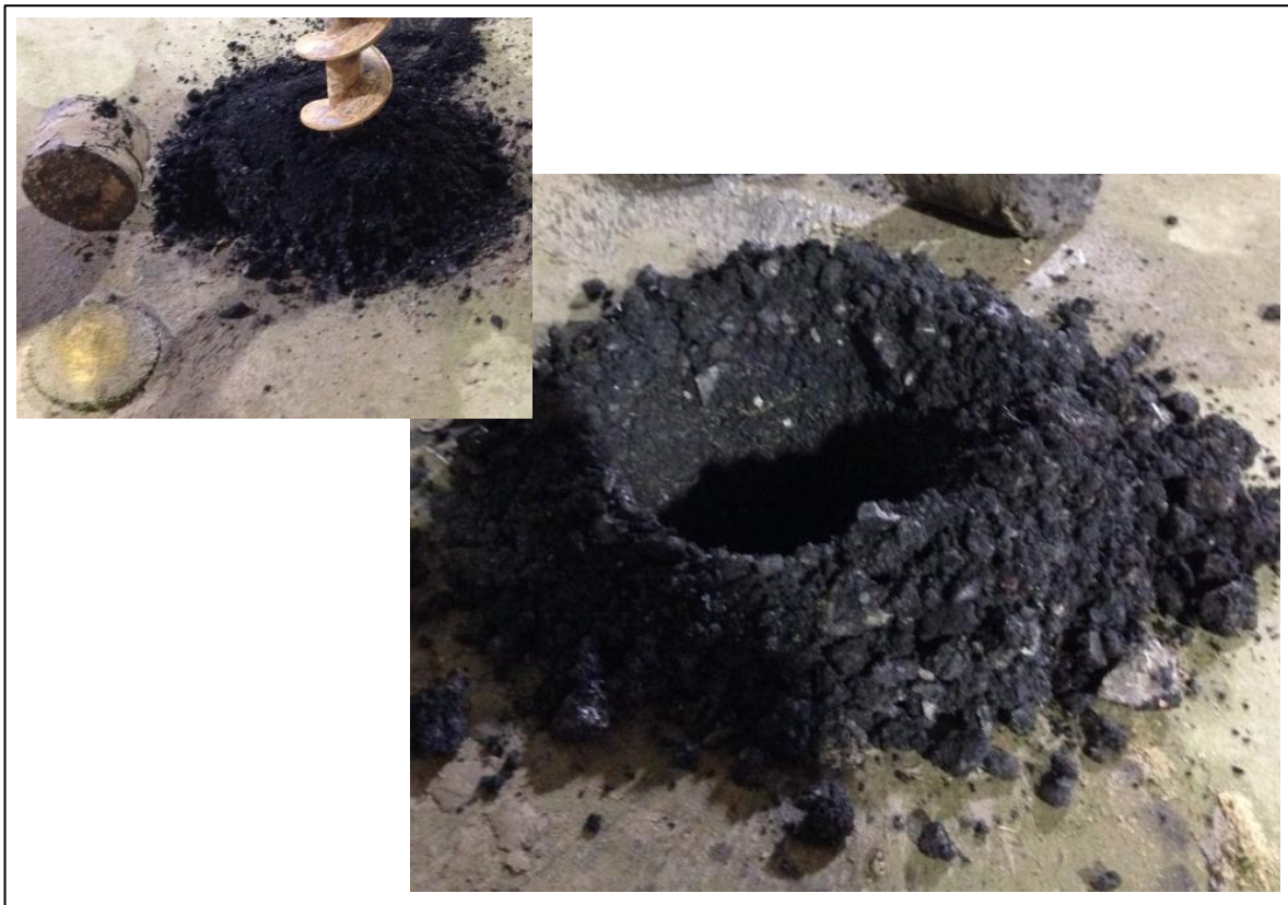
Photograph 3: Coalwash fill below cemented slag in each of the boreholes drilled.
